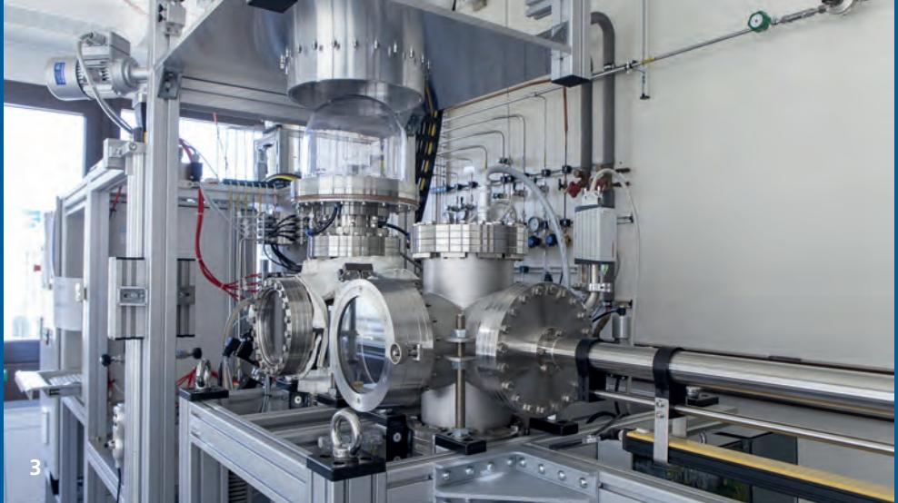
**3 Growth reactor that can be loaded with up to 600 diamond seeds or a single 6" wafer.**
