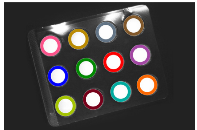
The 12 tablets are optically scanned and classified within 0.3 seconds.
