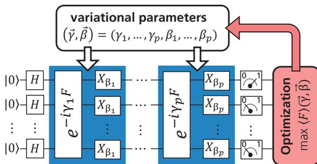
Quantum circuit of the QAOA algorithm with classical optimization of the parameters  $\vec{\gamma}$  and  $\vec{\beta}$  © Fraunhofer IAF
