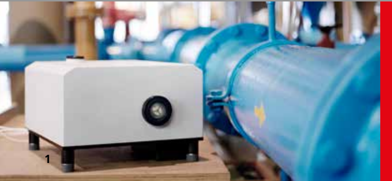
1 Just a little larger than a shoebox: the demonstrator analyzes water samples at the waterworks itself.
