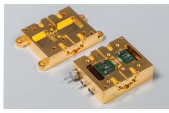
Medium power amplifier (MPA) for use in E-band, developed at Fraunhofer IAF
